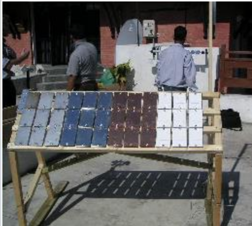
Corrosion monitoring track installed in Kathmandu, Nepal
